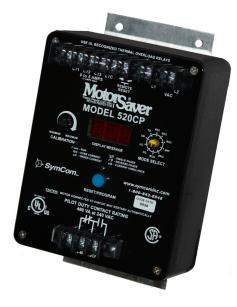
SymCom's Model 520CP is a fully programmable, microcontroller-based, current sensing device designed to monitor 3-phase pumps or systems with ramp up times of 4 seconds or less. Applications include submersible pumps, booster pumps, reverse osmosis systems, centrifugal pumps, vertical turbine pumps, oil well pumps, chemical pumps or other similar systems.
